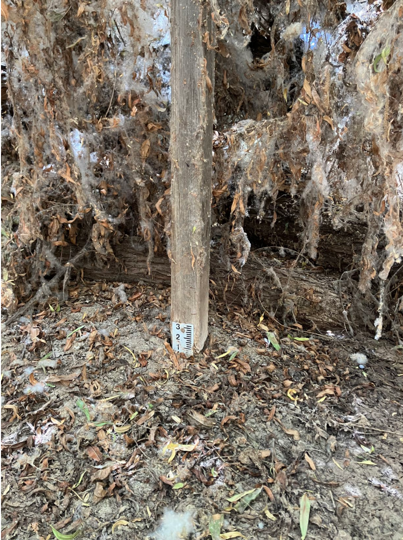
Figure 13. Photo of the SED 2 sediment gauge at Cottonwood Wetland reaching its measuring capacity. Photo was taken in the 3 rd quarter.
